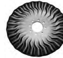
20VT-COMBO 20" Dia Z-shaped flutes 25 flutes, 1/2" overall 8 bolt holes 3-7/16" center hole
